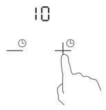
3. When the time is set, it will begin to count down immediately. The display will show the remaining time and the timer indicator will flash for 5 seconds.
